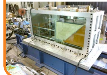
Conducting a shaking table experiment
