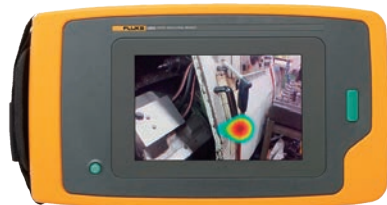
Air leakage diagnostic
